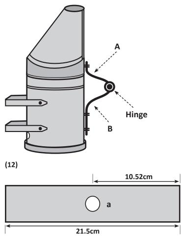
(i) Cut 2 pieces of plyan wire and make a rivet hole in the middle
