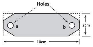
Fig 46: Measurements and making of a bee smoker:
