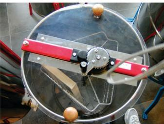
Fig 31: Centrifuge extractor
