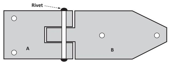
(9) Fix the part of No. 4 to part of No. 7 with a hinge above.
