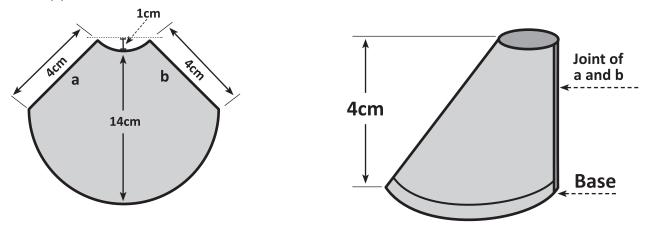
(iii) Fold out the base 2 mm at right-angle to the base of the cone
