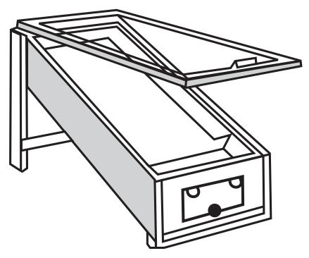
Fig. 63: Sketch of a solar wax extractor
